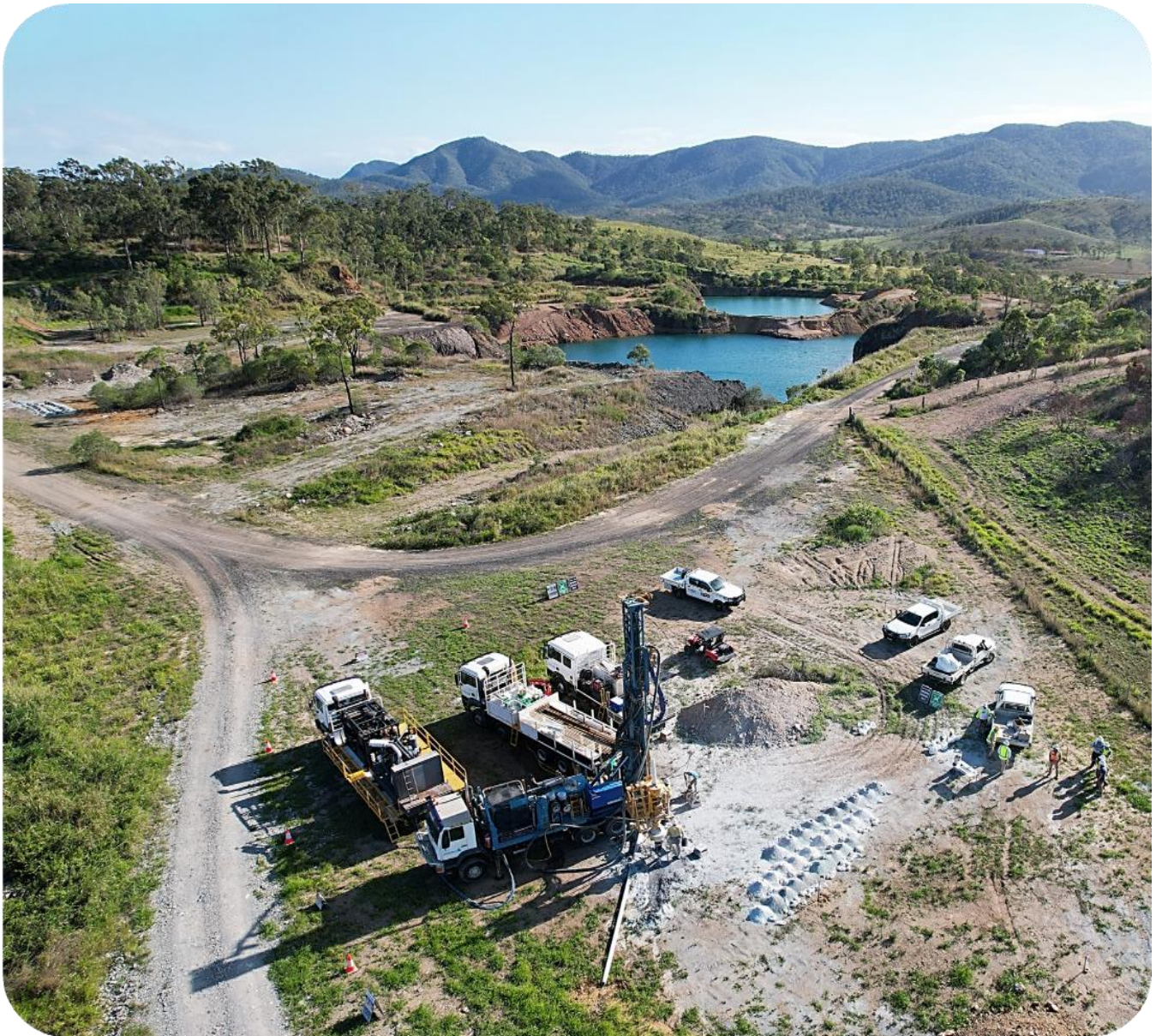
Figure 8: RC drilling at Mt Chalmers, 2023.
