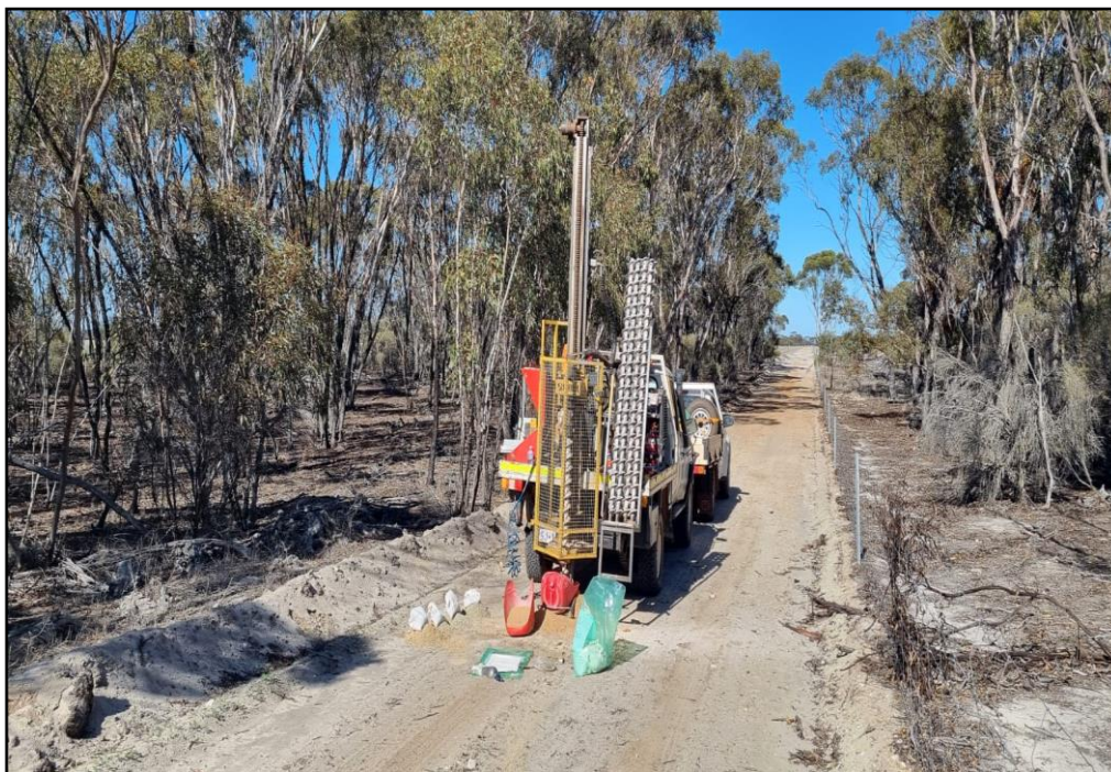
Figure 6. Auger Drilling at ZMI's Cascade Project, May 2024.
