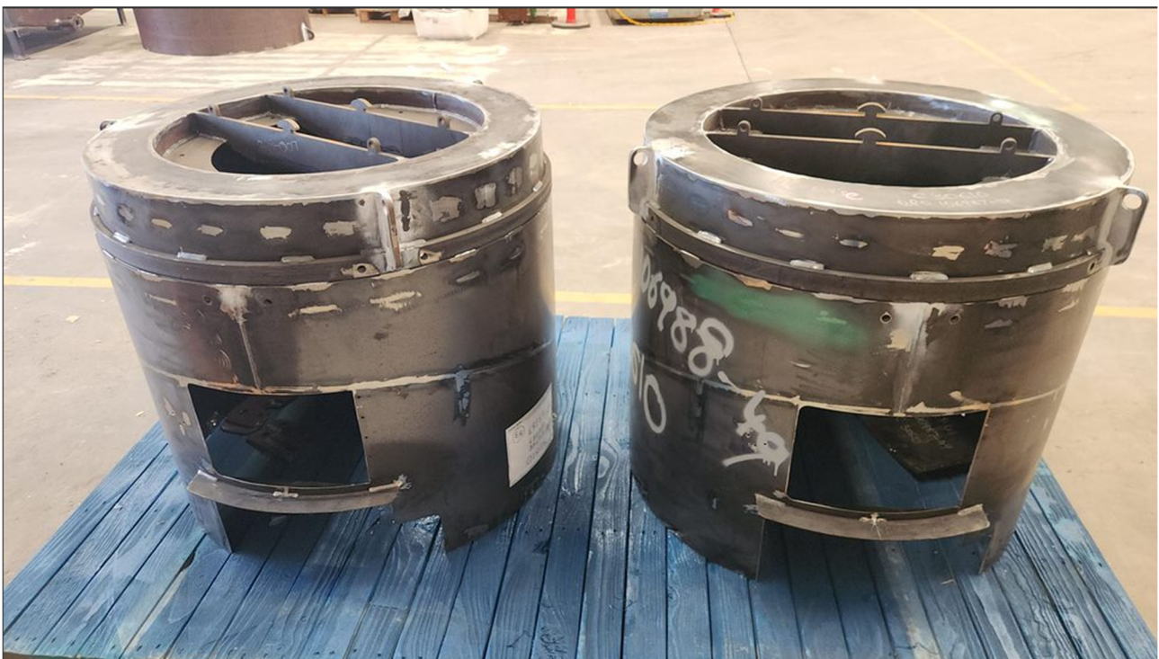
Figure 12: Knelson concentrator fabrication completed; rubber lining and painting underway.
