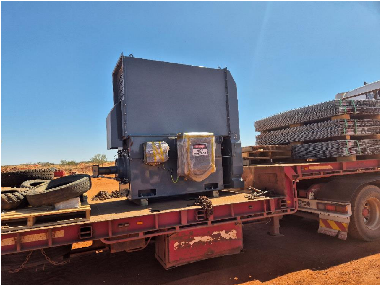
Figure 11: Refurbished ball mill motor delivery.
