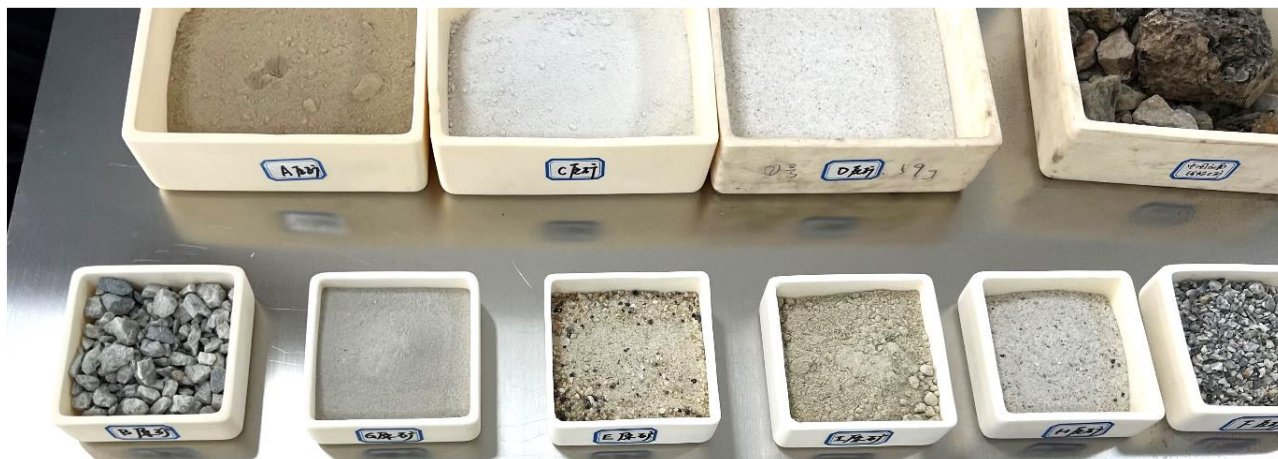
Figure 12: Various Spodumene Concentrates from around the world showing various particle sizing and grades
