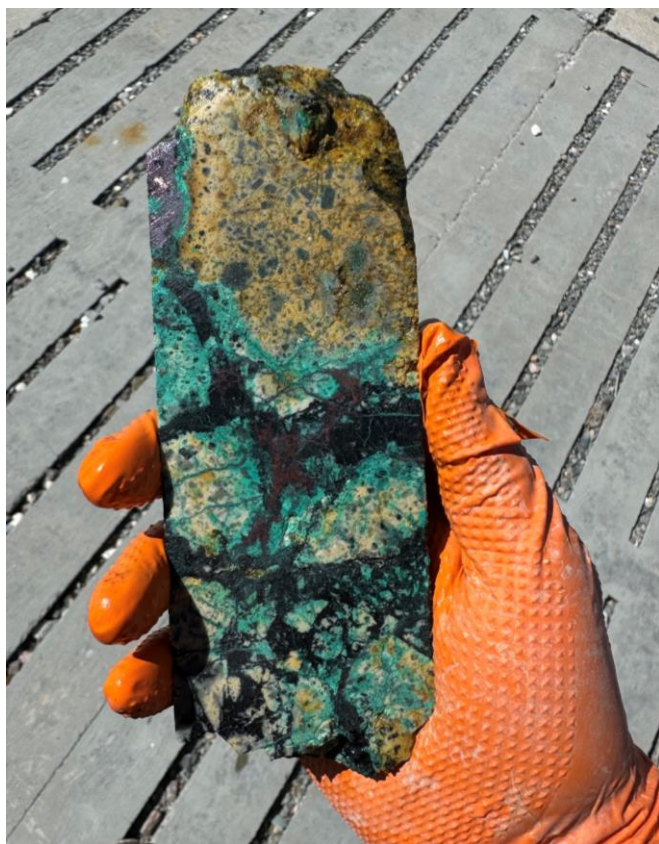
Figure 2: NY2024-DDH2 drill core at 14.0-14.2m downhole. The pXRF copper grade over 3 readings averages 23.2%.
