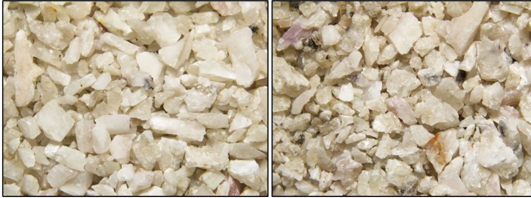
Figure 8: HLS concentrate fractions grading ~6.0% Li 2 O (left) and ~5.5% Li 2 O (right)
