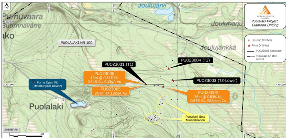
**Figure 6:** Map showing the location of the Avira diamond drillholes with significant intercepts and historic gold mineralisation.
