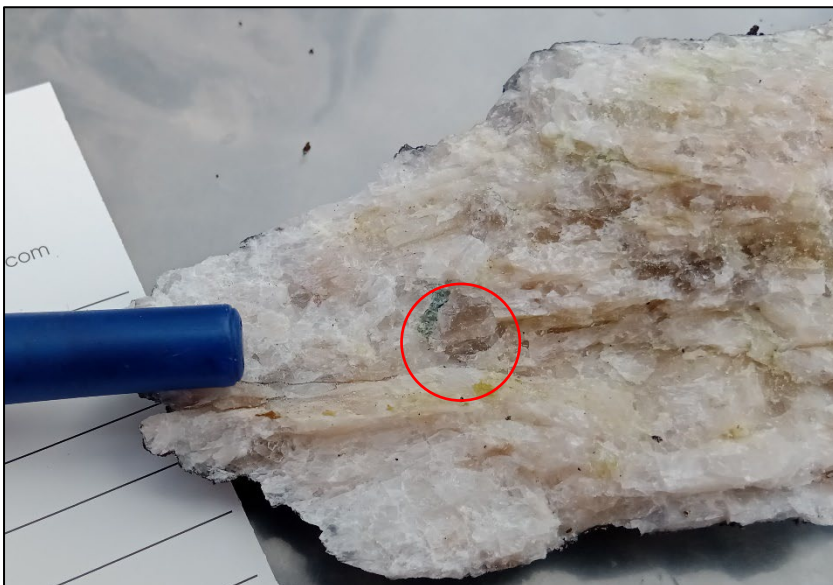
Figure 15 and 16: Left: Pegmatite containing potential beryl ( \pm Apatite?) mineral within Dalmas project (Pen lid for scale, 316859mE, 5943604mN, WGS 84/UTMZ19N), Right: Quartz Feldspathic pegmatite sample taken from Hiver project (302519mE, 5995547mN, WGS 84/UTMZ19N)
