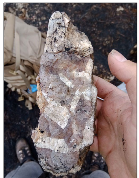
Figure 15 and 16: Left: Pegmatite containing potential beryl ( \pm Apatite?) mineral within Dalmas project (Pen lid for scale, 316859mE, 5943604mN, WGS 84/UTMZ19N), Right: Quartz Feldspathic pegmatite sample taken from Hiver project (302519mE, 5995547mN, WGS 84/UTMZ19N)
