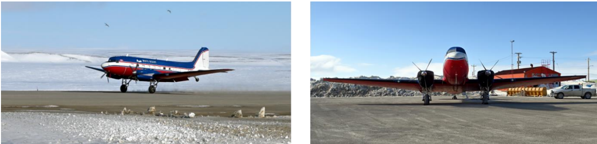
Figure 2. Basler BT-67 at Rolute Bay Airport to undertake geophysical survey for Somerset.
