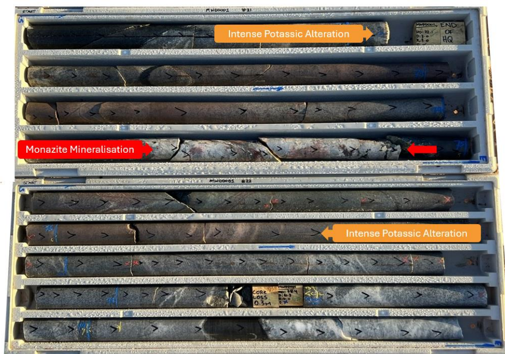
Figure 4: MWDD01 structurally controlled monazite veining from 74.1 – 74.9m within intense potassic alteration halo. The mineralisation represents a new REE mineralisation lode not observed at surface.
