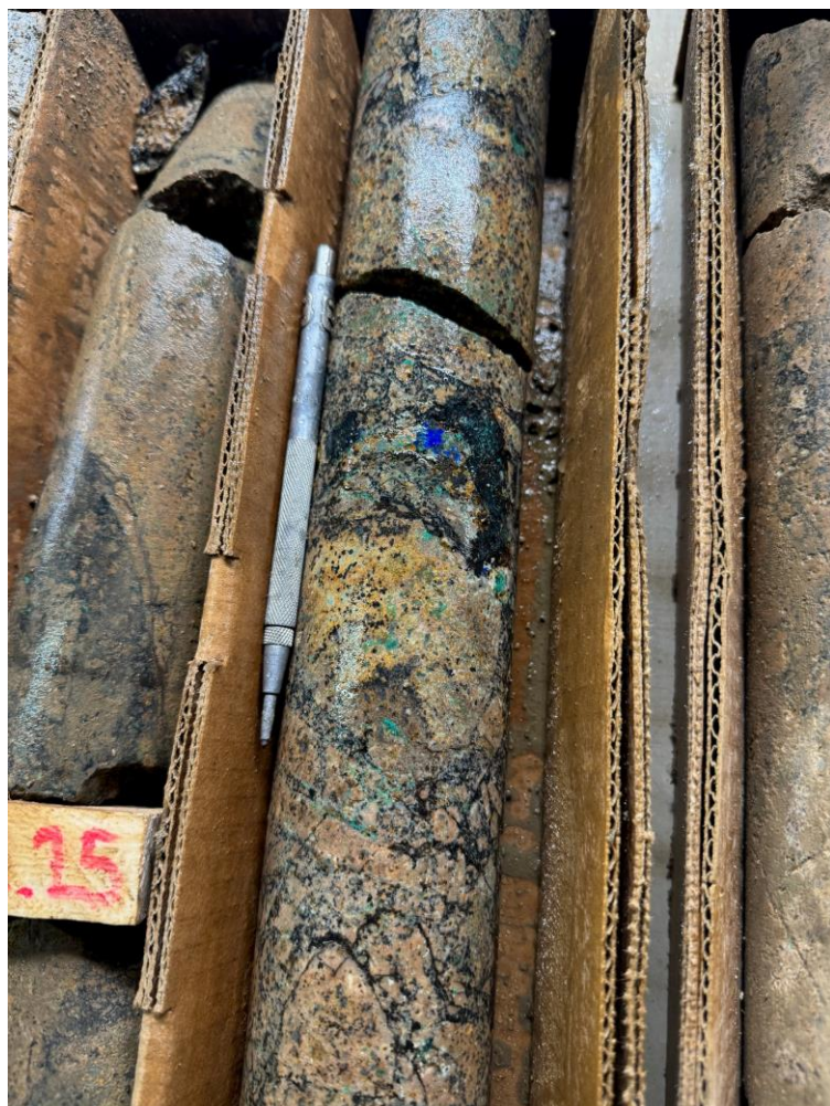
Figure 4: Disseminated malachite (green) and azurite (blue) copper oxide mineralisation at 22-23m down NY2024-DDH3. Averaged pXRF assays in this interval grade 3.2% copper.
