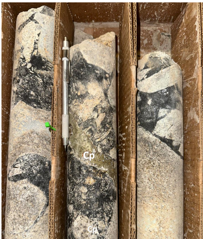
Figure 2: Chalcopyrite (Cp) in tourmaline breccia between 74.0-76.0m down NY2024-DDH3. The averaged pXRF copper grade over 3 readings for the interval is 10.0%.
