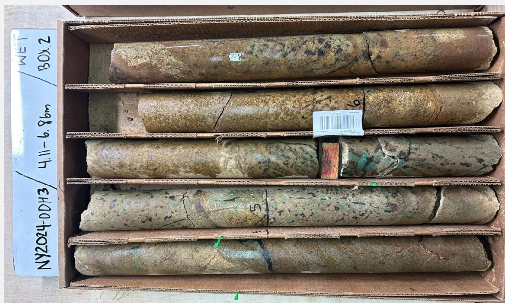
Figure 1: High grade copper mineralisation in tourmaline breccia in hole NY2024-DDH3. Spot pXRF grades range up to 8.0% copper within the interval from 4.5-5.5m.
