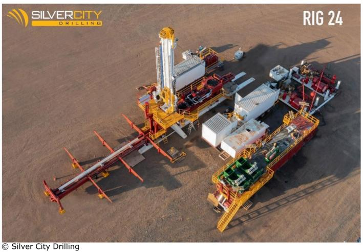
**Schramm T200XD Top Head Drive** Static Hook Load 200,000lbs / Hydraulic Pulldown 32,000lbs
