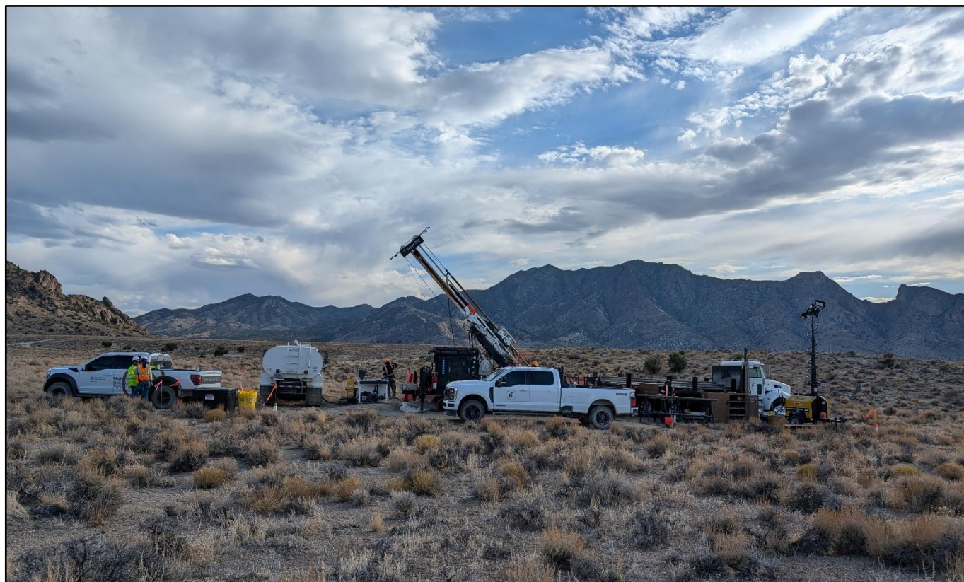
Figure 1. True North diamond drill rig set up at site RMS024.
