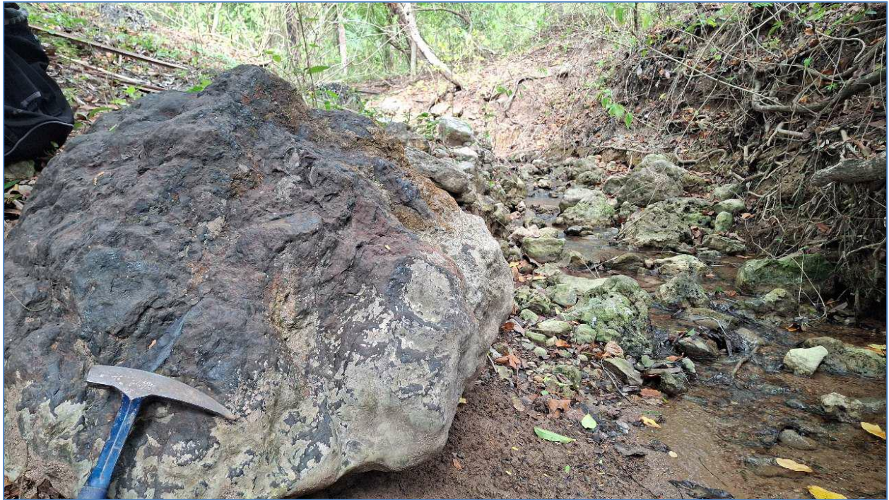
Figure 4: Subcropping chert and supergene material (estimated 85% chert, 15% manganese oxides) near the Sica Prospect This was not submitted for assay however pXRF readings from the manganese oxides were around 21% Mn indicating strong supergene enrichment. Cautionary Statement of pXRF – portable XRF results that are announced in this report are from uncrushed, rock-chip samples and are preliminary only. The use of the Bruker Titan S2 pXRF is an indication only of the order of magnitude of expected results.
