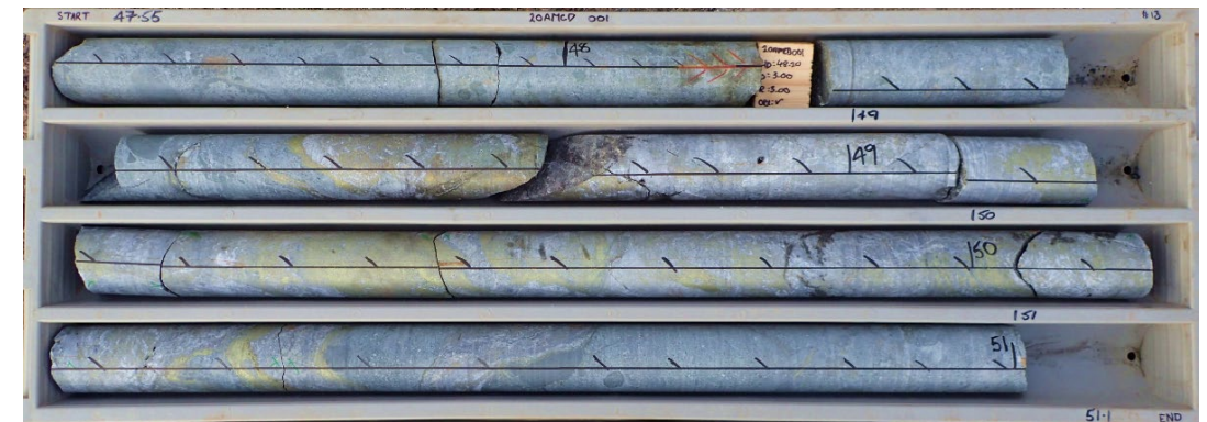
Semi-massive to stringer chalcopyrite mineralisation at Mons Cupri within chiolite-altered Cistern Formation
