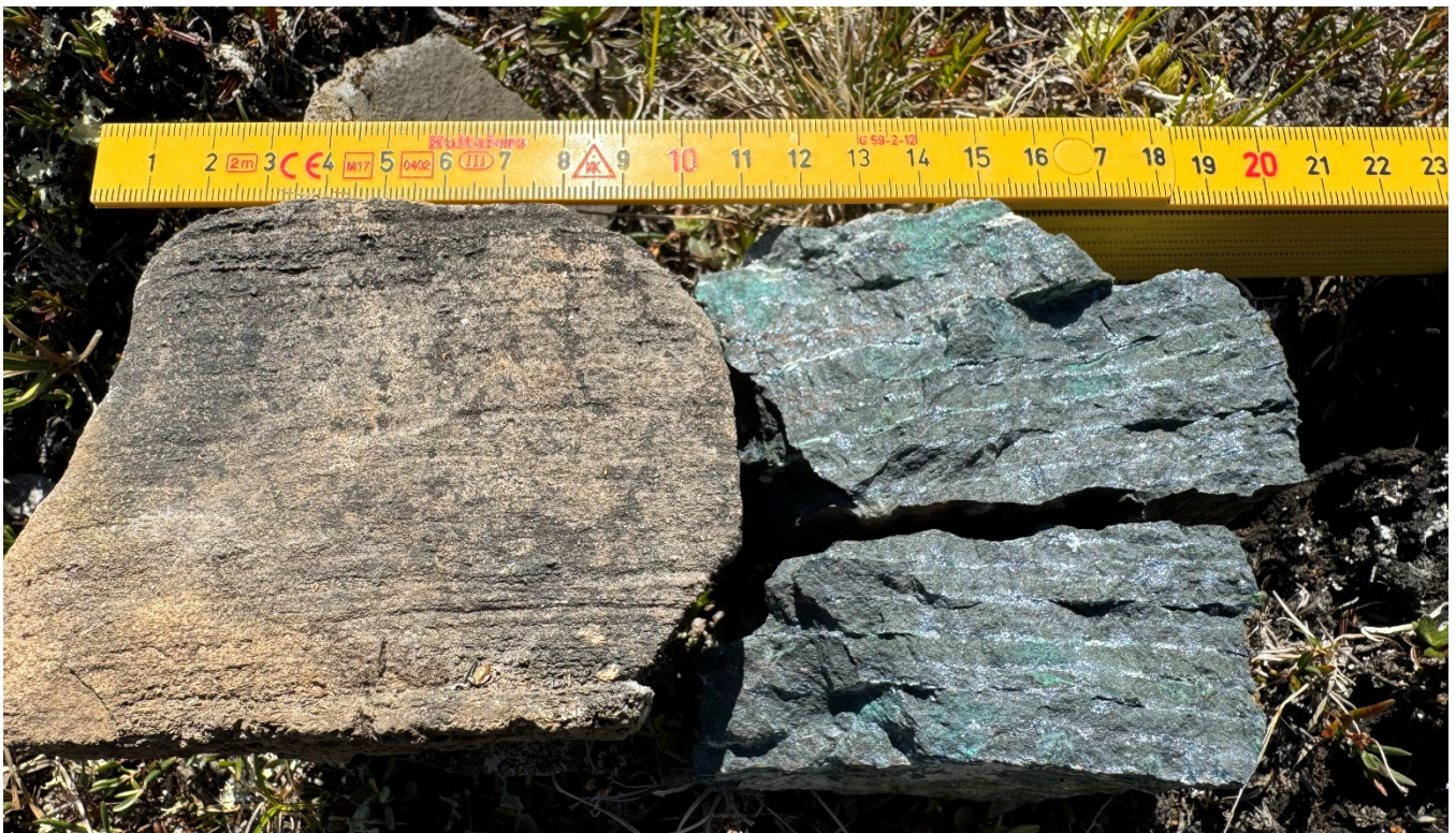
Figure 3: Photograph of sample F0005932 (right of image), a chalcocite replaced sandstone from the HALO target area which returned 23.8% Cu.
