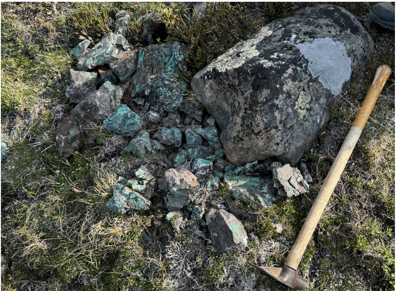
Figure 5: Photograph of outcrop sample F005937 from the Cu-TAR vein target within the Rocket exploration district which returned 37.3% Cu and 15g/t Ag .
