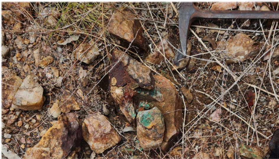
Figure 2. New San Quentin Prospect sub cropping copper mineralisation discovery, sample QL6982 pXRF reading of 3.5% Cu in quartz iron oxide breccia.
