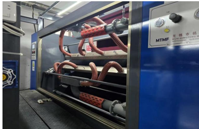
One of 31 Air Knives in Qunying Corp Factory (each requires two blowers)
