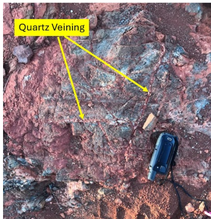
Figure 5: Location 3 showing quartz veining in mafic rock, GPS shown for scale (393766m E, 6790782m N). (Refer Figure 2 for physical location relative to tenement holdings.)
