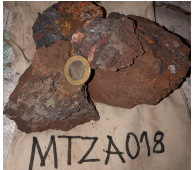
Figure 6: Gold mineralization assayed 17.5 (g/t) in Ferruginous Quartz Feldspathic vein (Gossan)X
