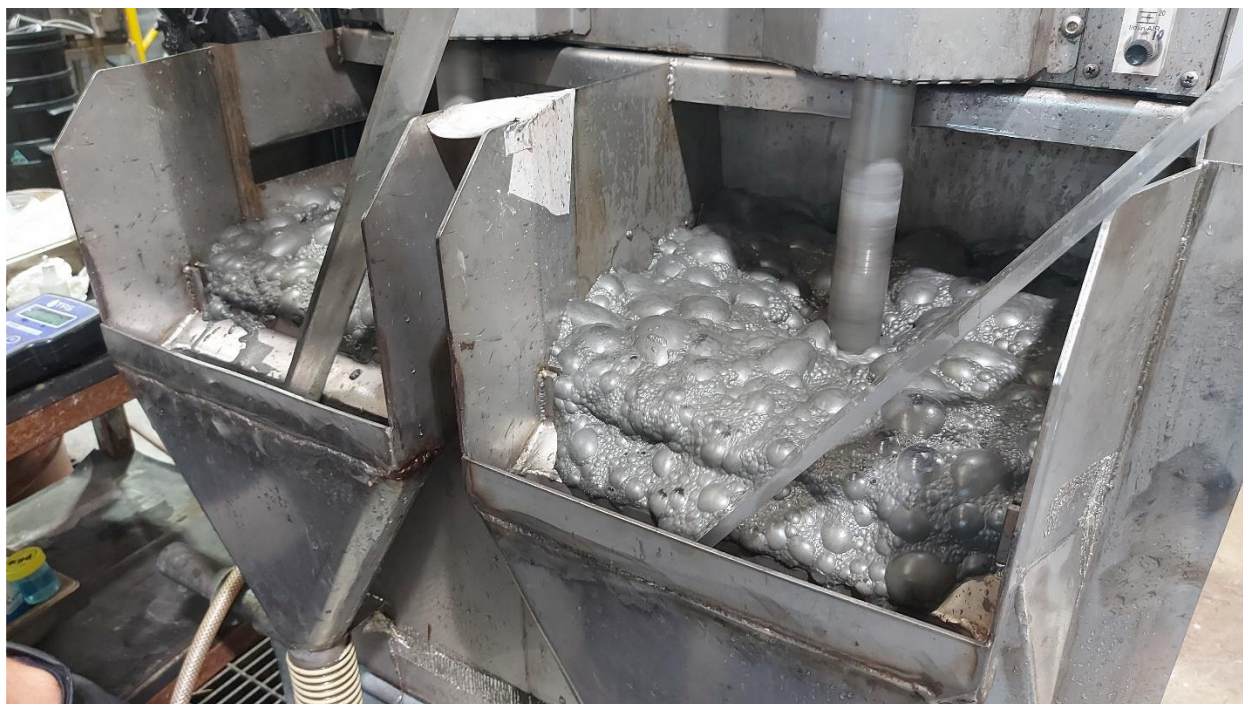
Figure 3: Photo showing sulphide flotation testwork being undertaken on the non-magnetic tail.
