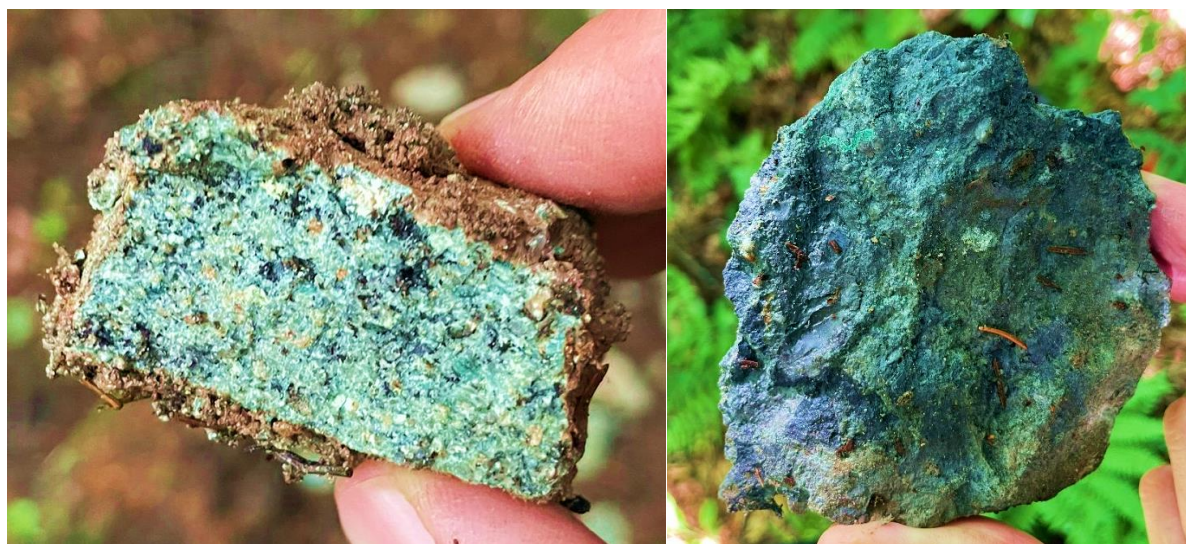
Figure 1. (Left) Sample of malachite-chalcocite altered sandstone grit that assayed 0.89% Cu (K031159) from Demoiselle; (right) Sample of malachite-chalcocite altered fine grained conglomerate that assayed 0.91% Cu (K031171) from Lower Cape.
