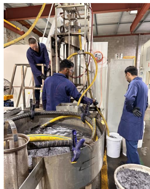
Figures 1& 2: Pilot-scale flotation at the third-party testing facility in Australia
