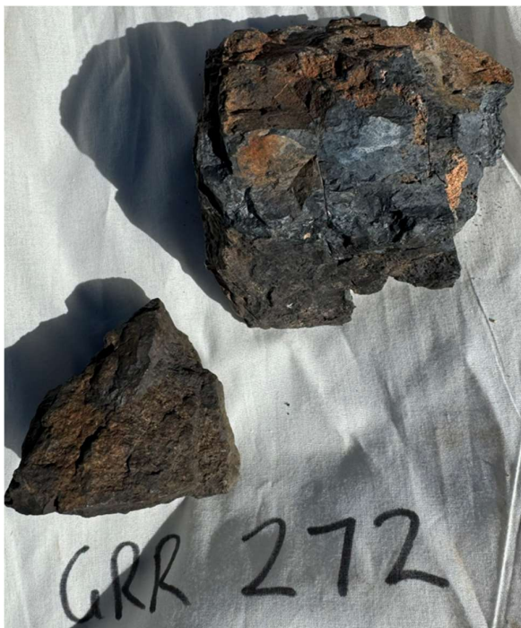
Figure 2: High-grade massive black manganese oxide mineralisation, 54.50% Mn, Sample GRR272
