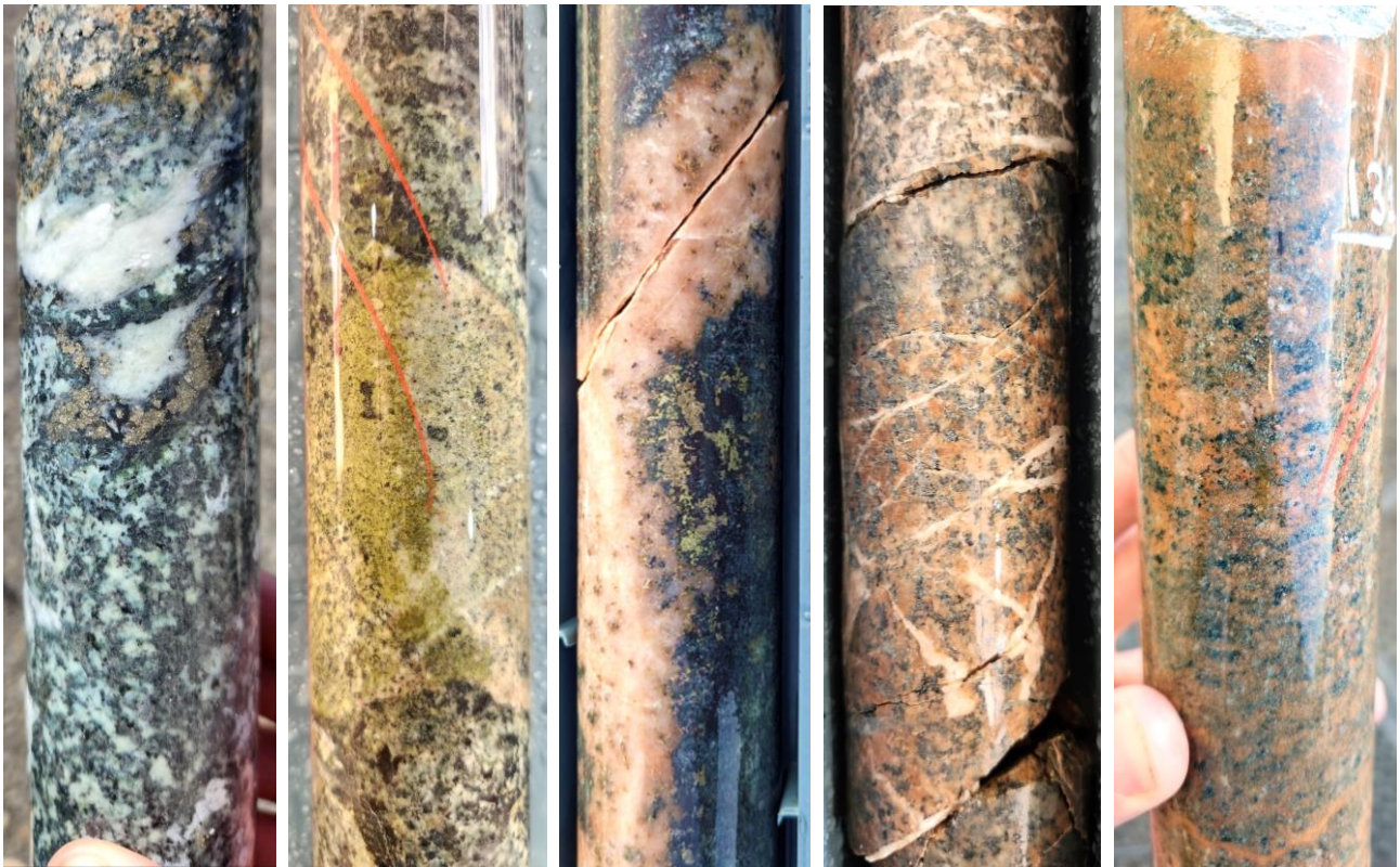
Figure 5: Examples of (left to right): chlorite-epidote-pyrite alteration, epidote alteration, quartz veining with pyrite-chalcopyrite, “redrock” (albite-hematite) alteration with carbonate veining, and redrock alteration with disseminated pyrite.
