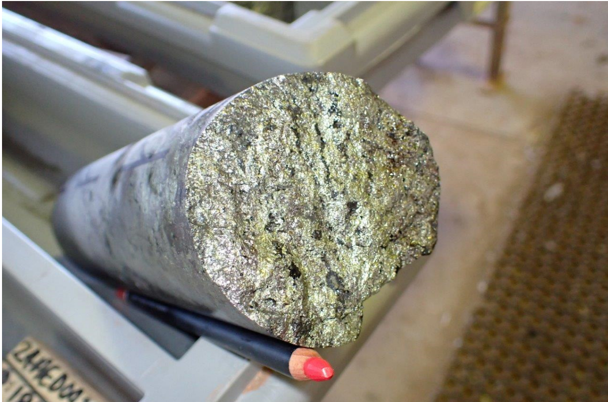
Figure 4: Massive sulphide mineralisation in 24AED002A
