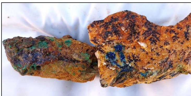
Figure 4. Sample PER015 collected near shallow unnamed workings at the southern end of the Black Ridge copper trend during reconnaissance mapping, showing secondary copper carbonates (blue and green) in a fractured limestone host and returning an assay grade of 6.5% Cu, 0.16g/t Au & 16g/t Ag (ASX MAG 1 August 2024).
