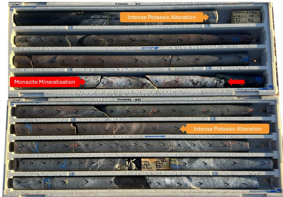
Figure 2: MWDD01 structurally controlled monazite veining from 74.1 – 74.9m within intense potassic alteration halo. The mineralisation represents a new REE mineralisation lode not observed at surface (see ASX:KFM 10 October 2024).
