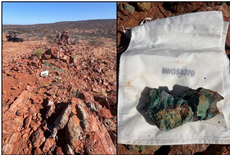
Figure 5: Ring Well surface sampling; MWGS3270 21.6% Cu looking Northwest. Mineralisation predominantly occurring as malachite with trace azurite and bornite (see ASX:KFM 10 October 2024).
