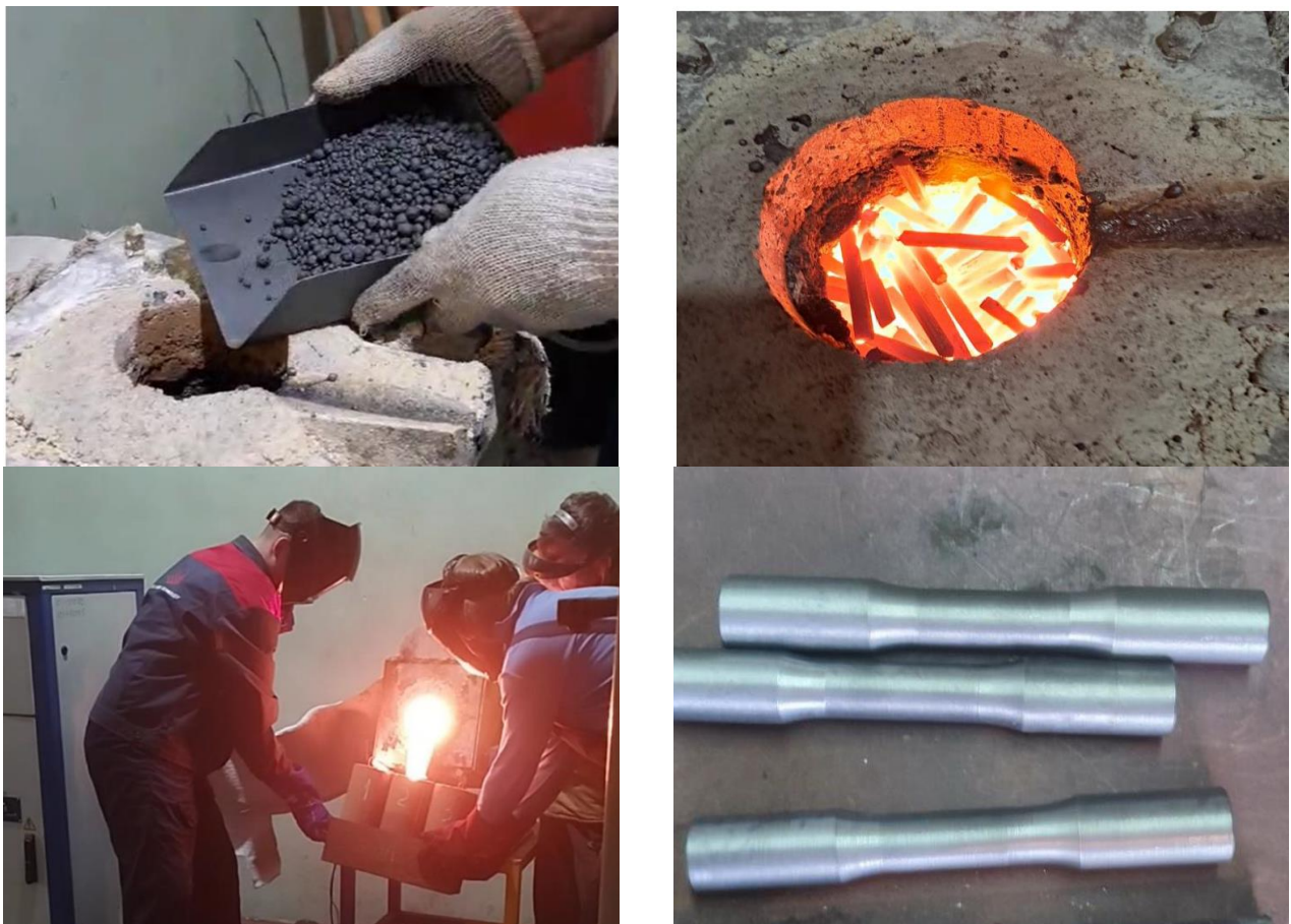
Figure 1 – Manufacture of Grey Cast Iron with Agglomerated Sarytogan "Micro80C" Graphite.
