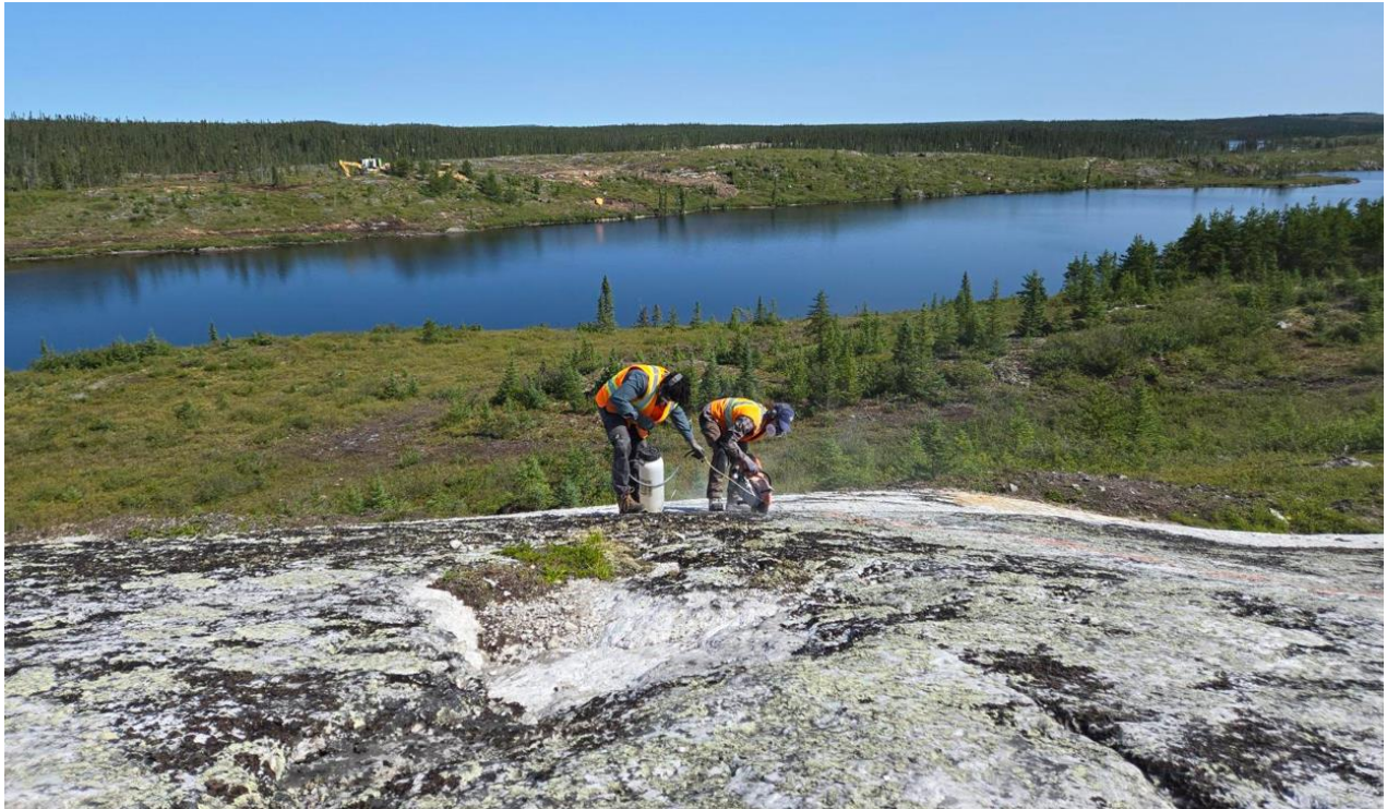
Figure 14: Channel sampling of the primary outcrop at the CV5 Spodumene Pegmatite.
