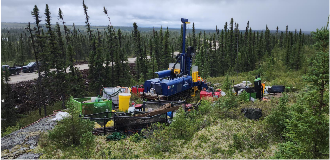
Figure 8: Geotechnical hole CV24-570 situated north of CV5 at a proposed infrastructure site.
