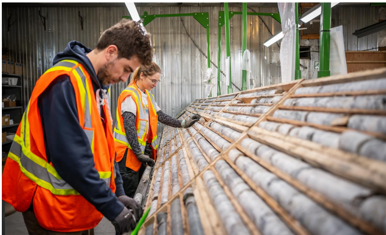
Figure 6: Drill core processing in core shack at site.
