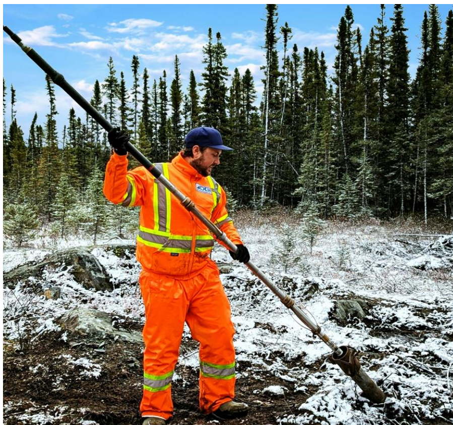
Figure 12: Televviewer survey instrument being placed in drill hole CV24-492.
