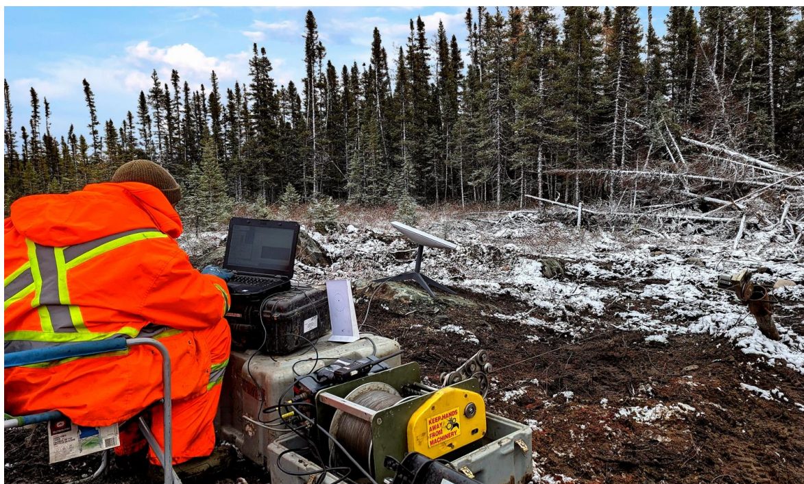
Figure 13: Televviewer survey data collection in drill hole CV24-492.
