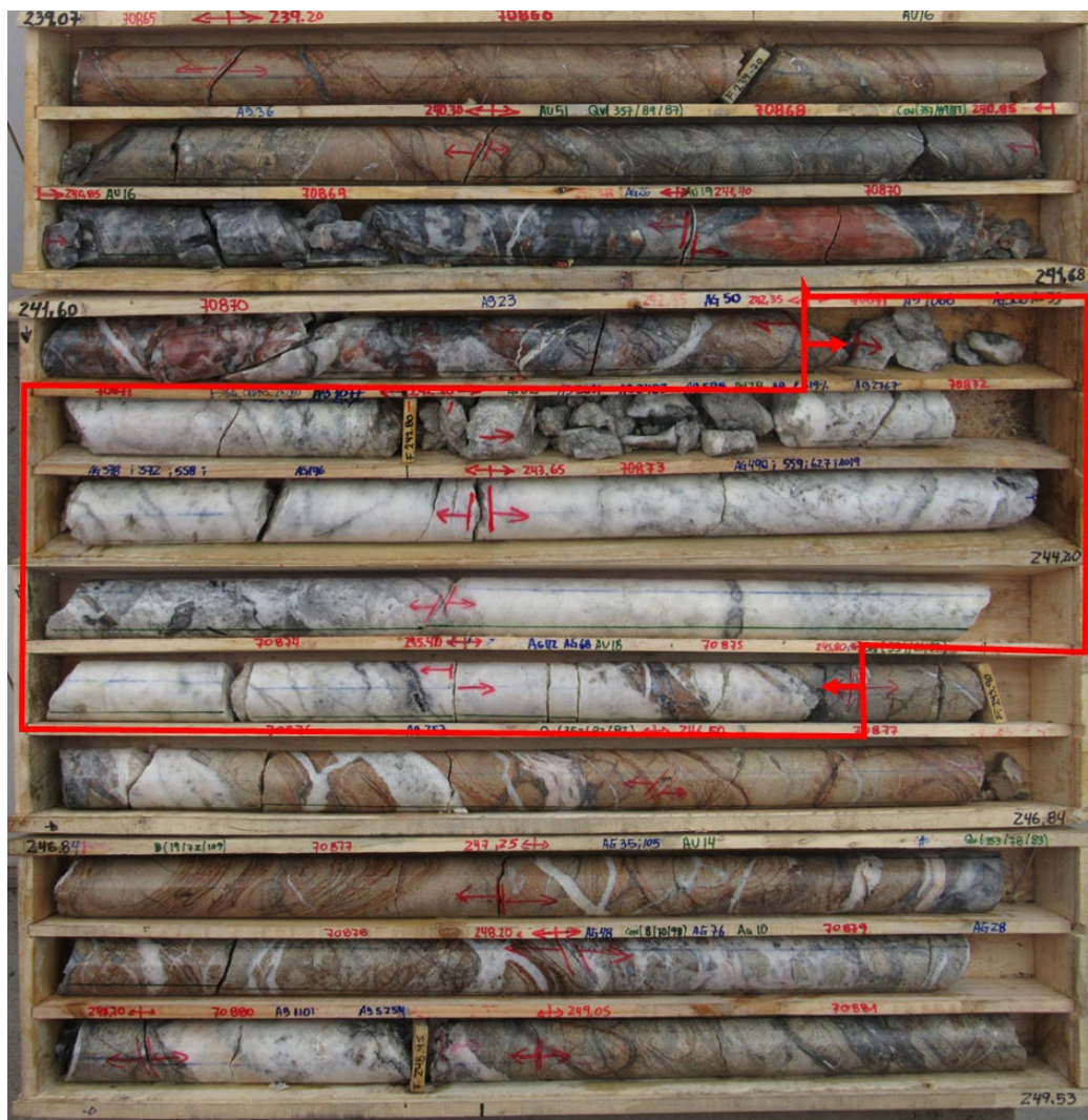
Figure 7. Hole CBD145 drill intercept of 3.1m @ 332g/t AgEq (192g/t Ag & 1.7g/t Au) hosted solely within a pre-mineral dacitic dome 3
