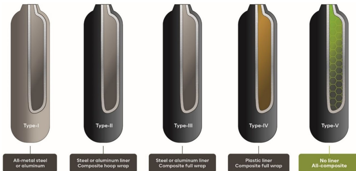
Figure 4: Five common pressure vessel types including the Type-V tank.
