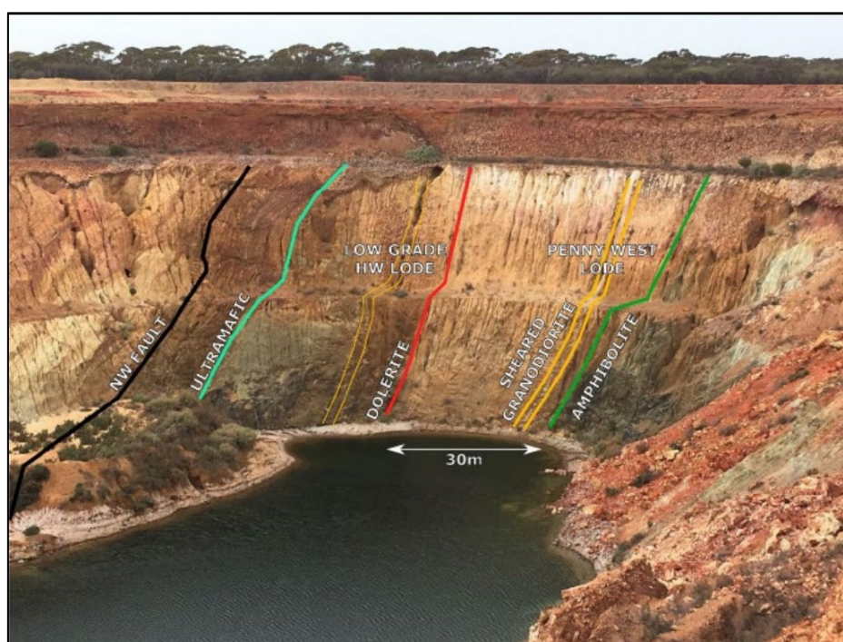
Figure 6: South wall of the Penny West pit (looking South) showing stratigraphic relationships to the Penny West Lode, noting high-grade and low-grade lodes (Source: ASX: Spectrum Metals Ltd, 29 August 2019)
