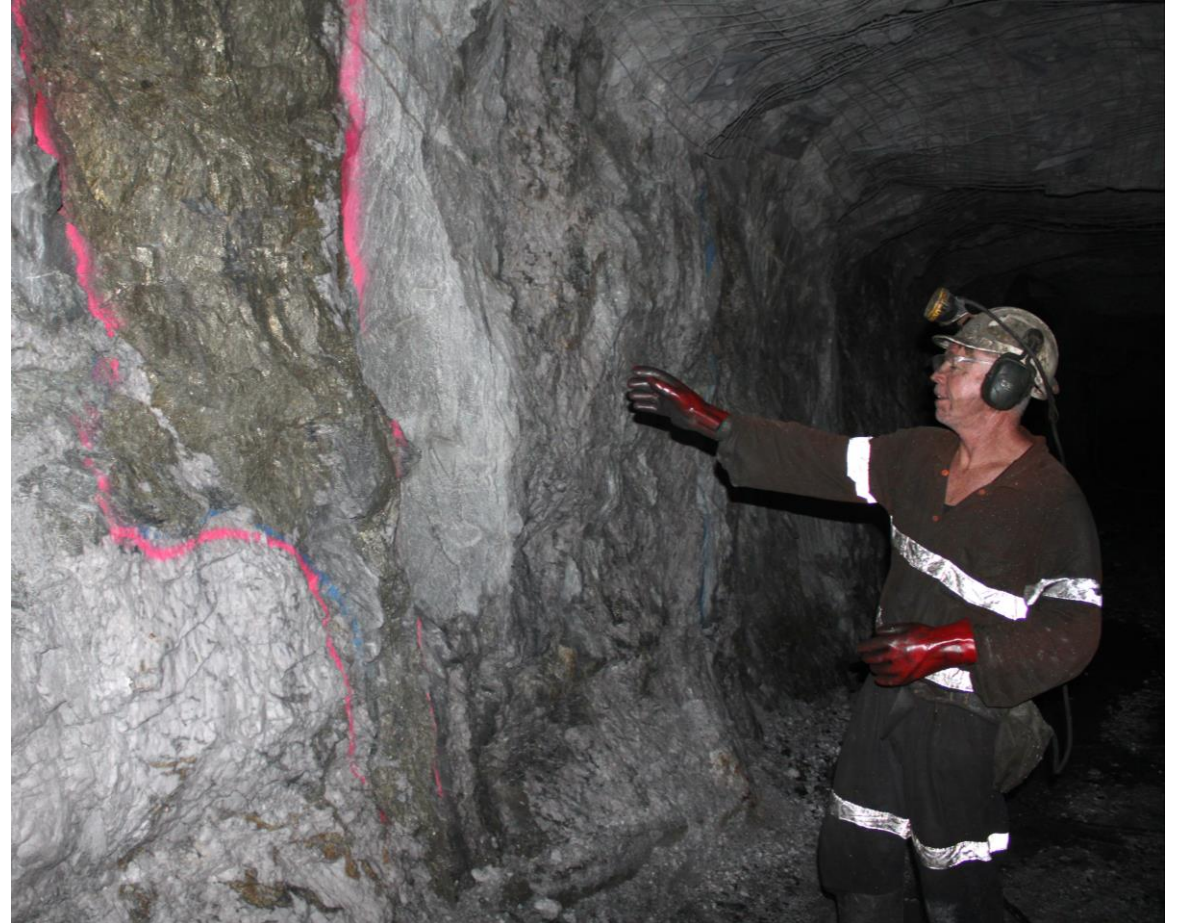
Cream mining lining up new drive turnout on 823 level at Paulsens
