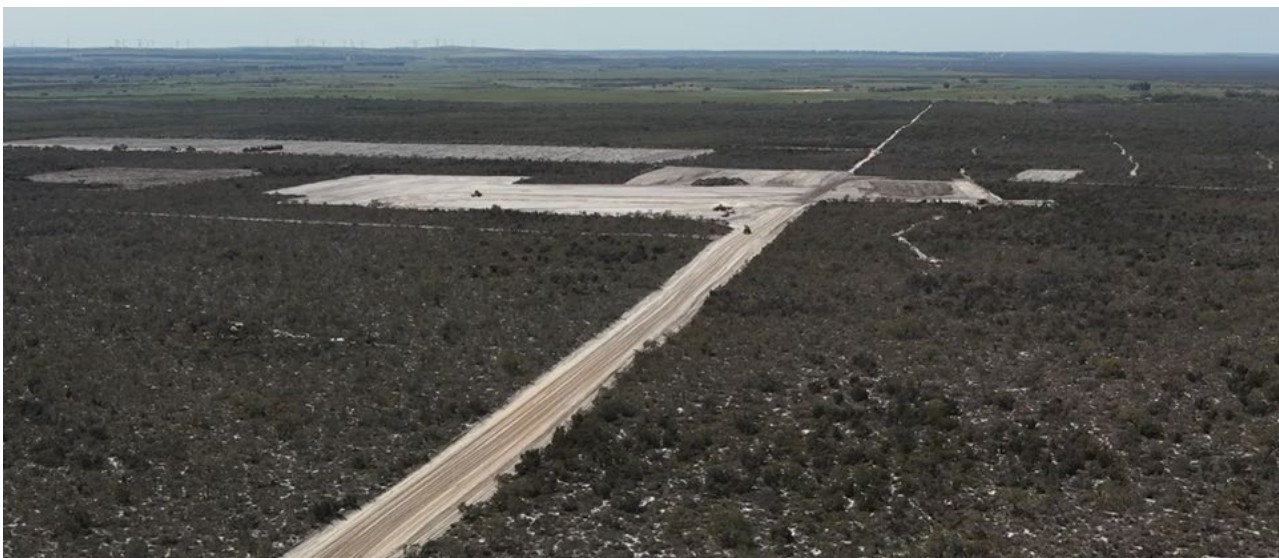
Photo 1: Atlas Mine – Access road and topsoil stripping
