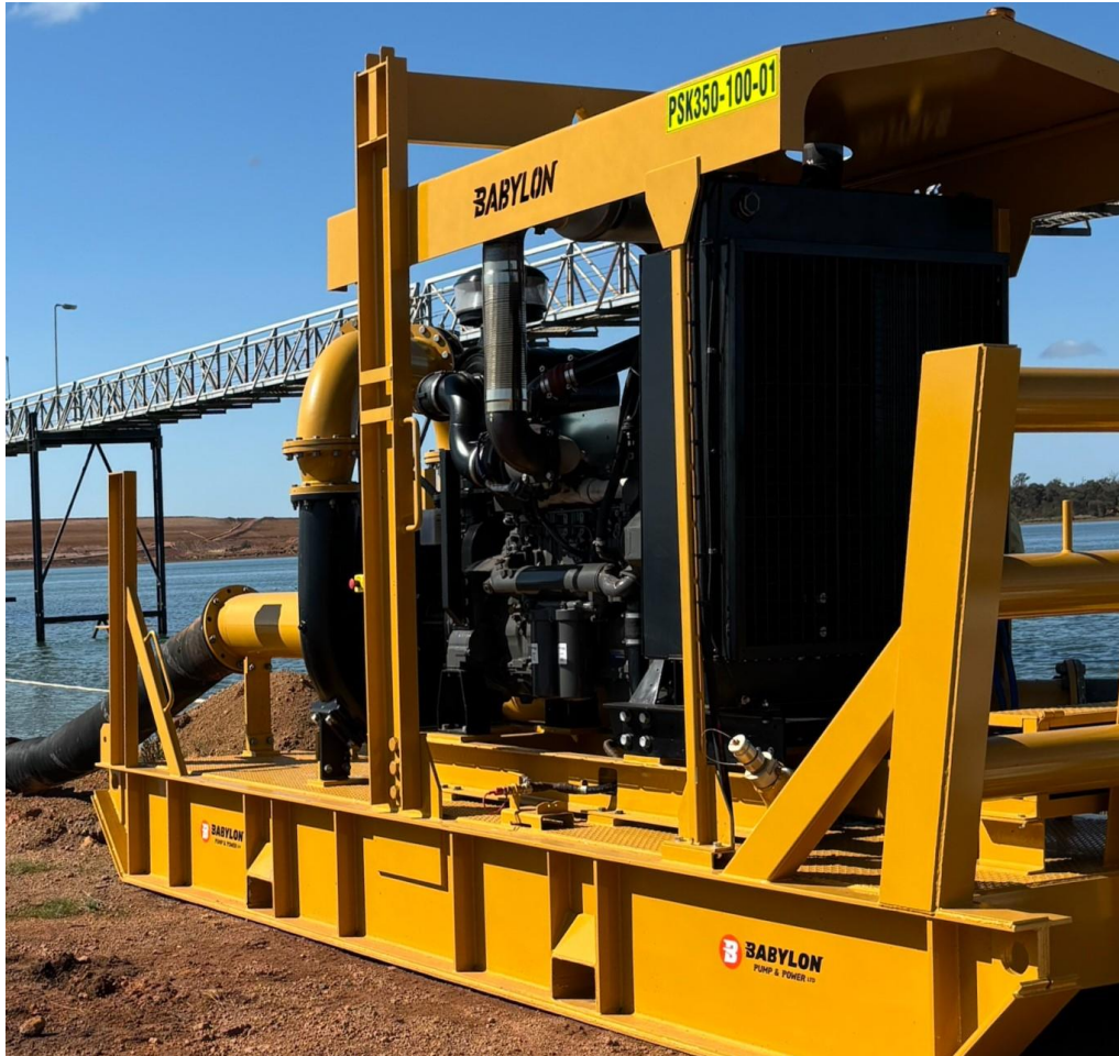
A Babylon high-flow pump recently installed at a major gold mine, capable of 350L/s at 100m head
