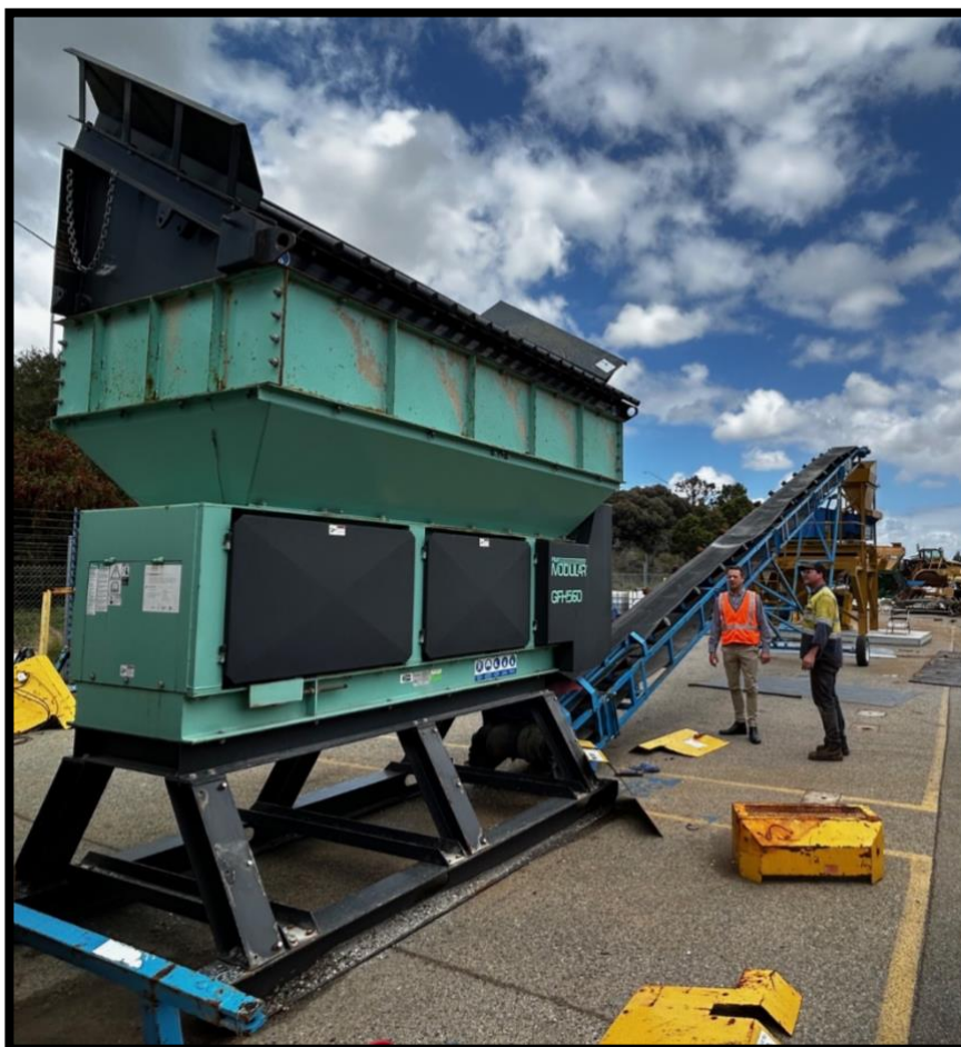
Figure 2: Feeder circuit of Gekko processing plant
