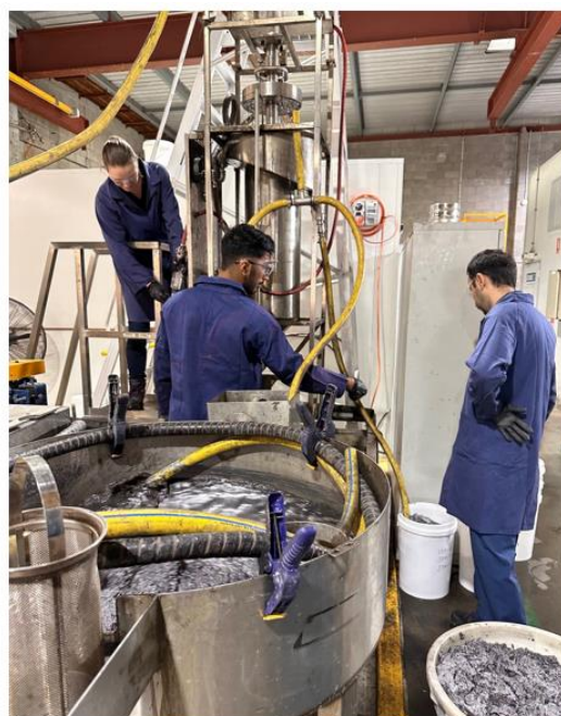
Figures 7 & 8: Pilot-scale flotation at the third-party testing facility in Australia
