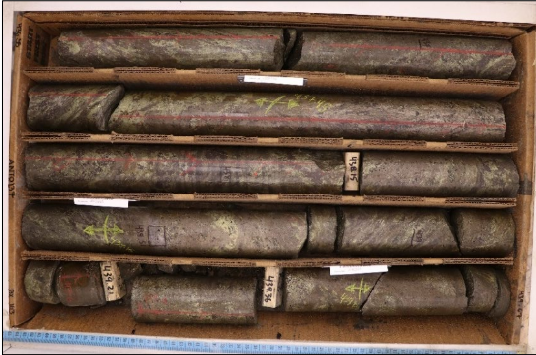
Figure 2 – ANT137 Massive Sulphide Mineralisation (436.55m to 439.67m)
