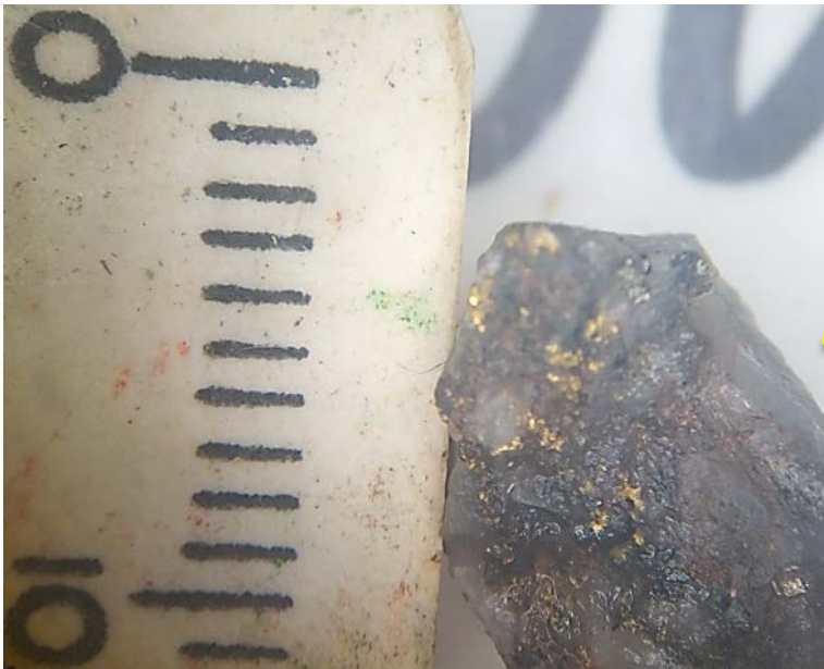
Photo of rock chip from hole TGRC23004, 117-118m sample interval with reported grade of 7.8g/t Au 2 . Scale on left is in millimetres (mm). See ASX Release 19 September 2023 for more details
