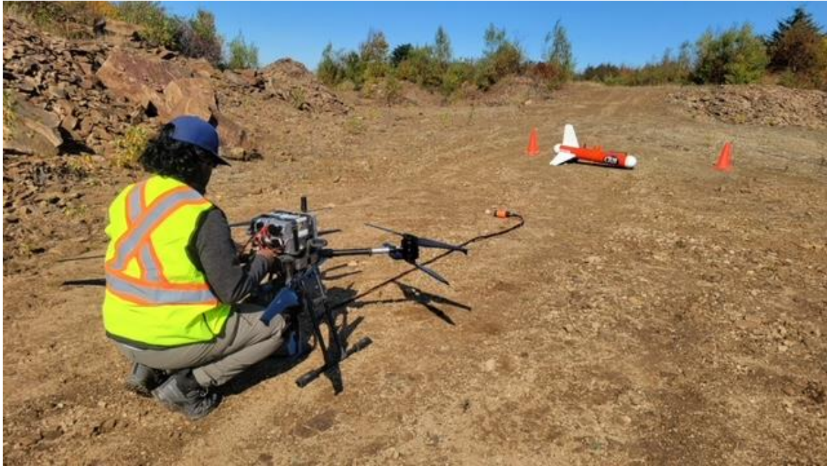
Figure 2. Pre-flight setup of UAV for aerial geophysical survey
