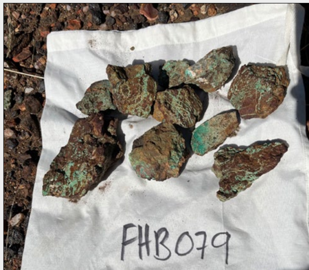
Chalcocite and malachite mineralisation – Sample FHB079 – Laboratory assays of 24% Cu and 0.14g/ Au.
