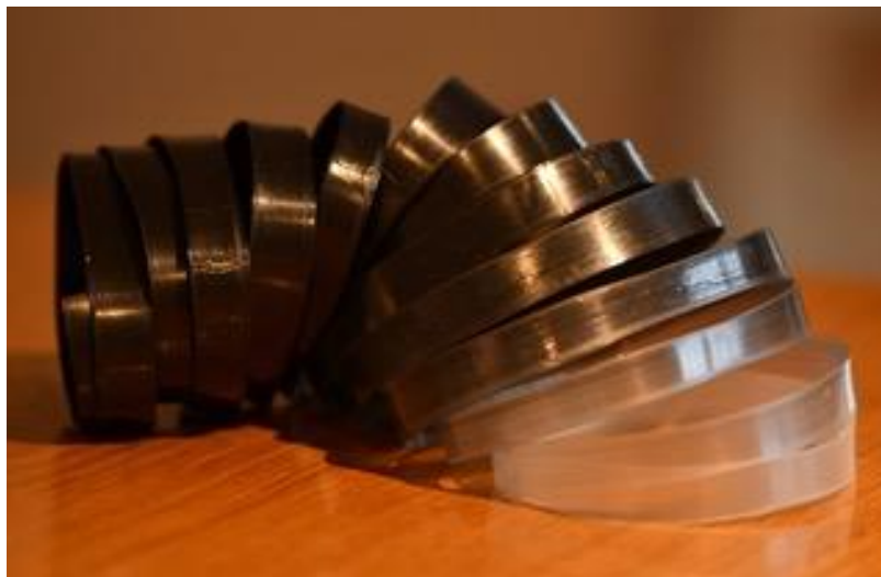
Polymer tape with progressively higher percentages of CNT added
