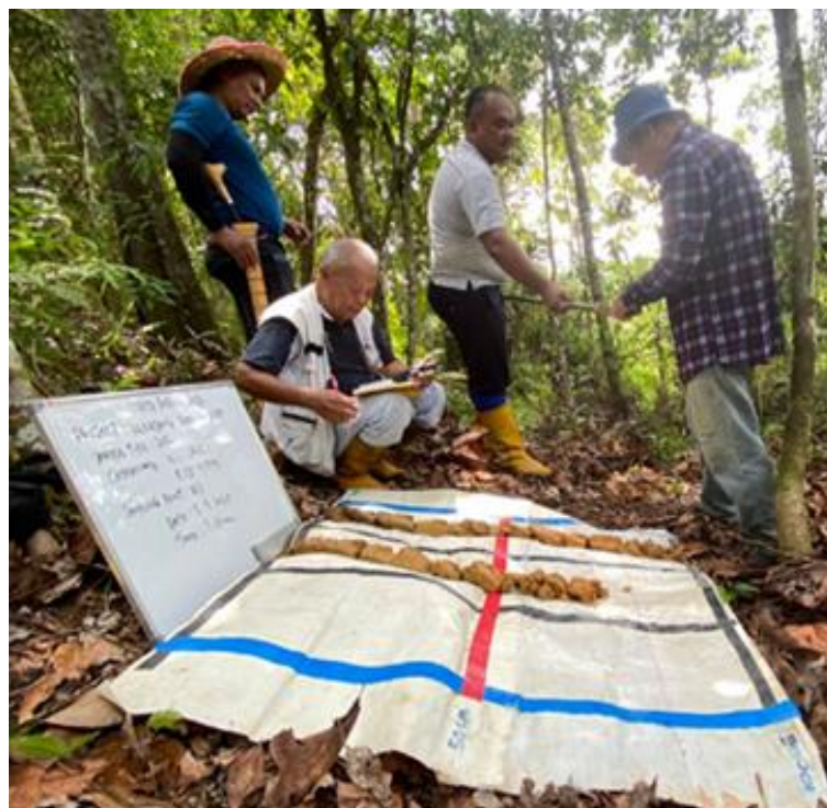
Figure 2 - sampling the soil profile at Bekajang for base-line contaminants.
