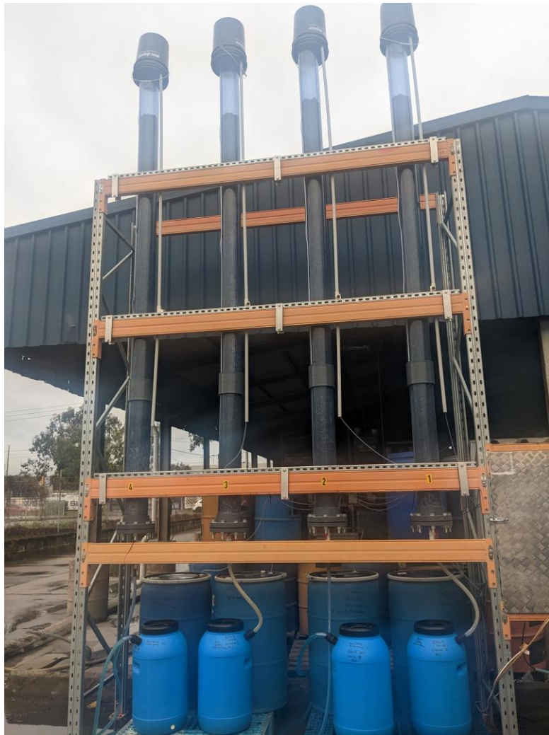
Figure 3: Column leach test work on Dianne Copper Deposit material in progress
