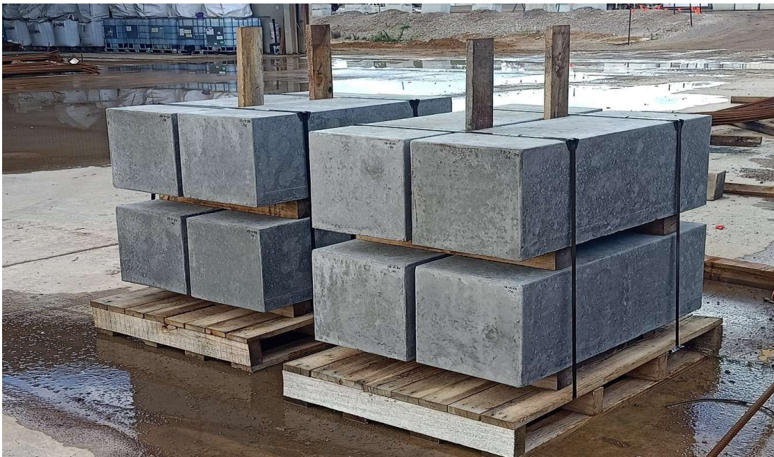
Figure: Low carbon backing blocks free from Portland cement
