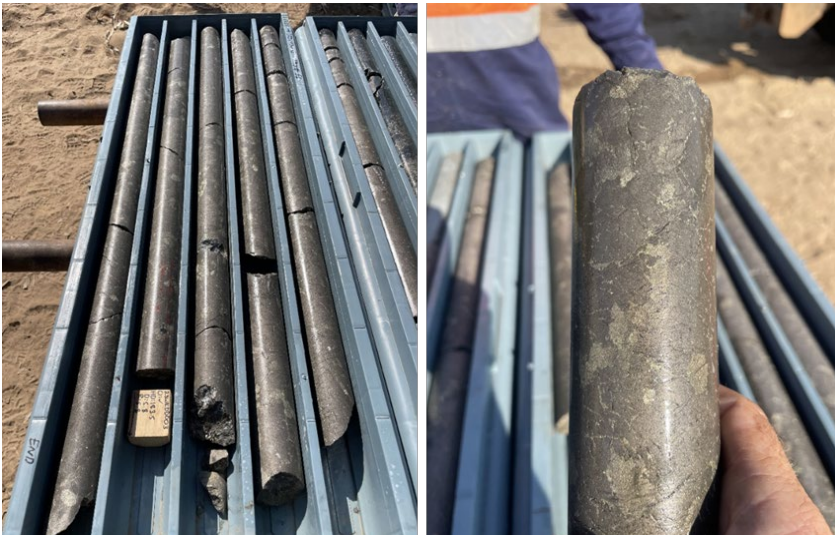
23WKDD003 at 179.1 m - massive sulphide mineralisation with visually logged Ni and Cu sulphides (ASX 4/10/2023)
