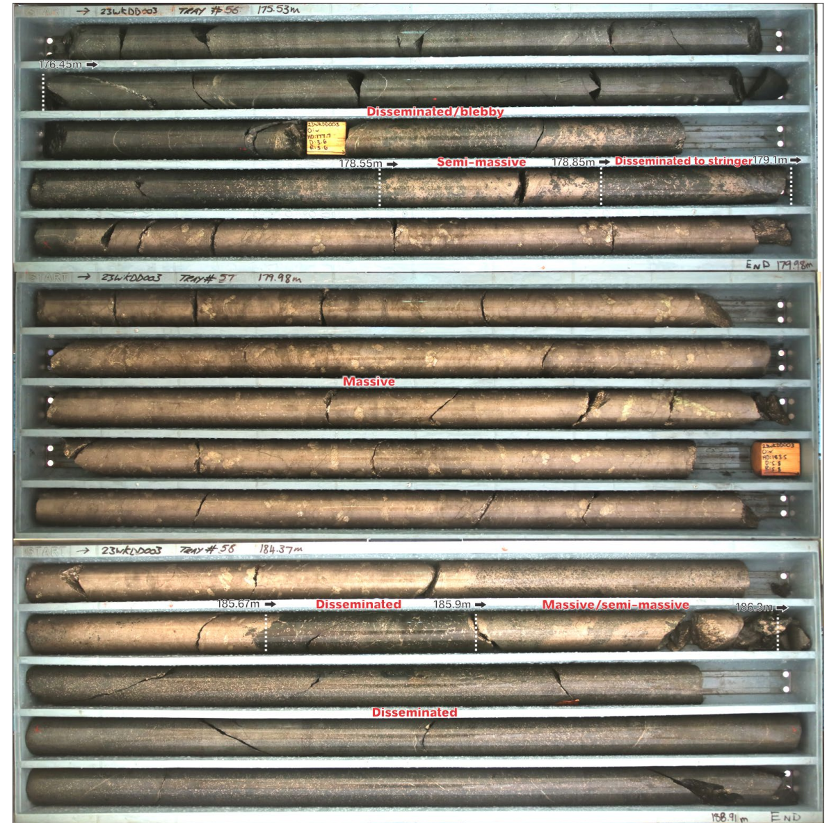
6.57 m of massive (>80%) sulphides intersected in hole 23WKDD003 at the Dogleg Prospect from 179.1 m, within a 14.7 m zone of mineralisation from 176.45 m (ASX 4/10/2023)
