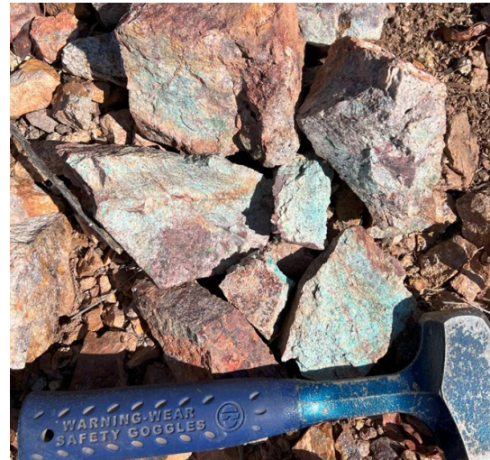
Sun Devil prospect sample DC0107 - 30,800 ppm (3.08%) Cu & 58 ppm Mo. Highly weathered ?Proterozoic intrusive rock with stockwork veining and supergene chrysocolla overprint. (ASX 11/03/2024)
