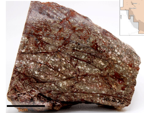
Leached plagioclase-phryic porphyry cut by quartz-iron oxide veins
