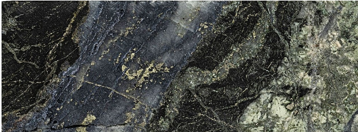
CPW0002DD at 619.70 m depth. The mafic schist on the left hosts a banded quartz-molybdenite vein which is cut by later veins of blebby sulphides. Disseminated sulphide is stronger in this mafic host compared with the chlorite altered felsic gneiss on the right of photo. Visually estimated sulphide abundances: 1.5% pyrite, 1.0% chalcopryite and 0.15% molybdenite. HQ3 core is 63.5 mm width. (ASX 06/09/2023)
