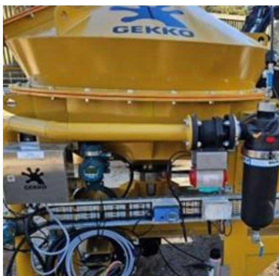
Figure 8: Wolff Batch Centrifugal Concentrator – coarse gold gravity collector
