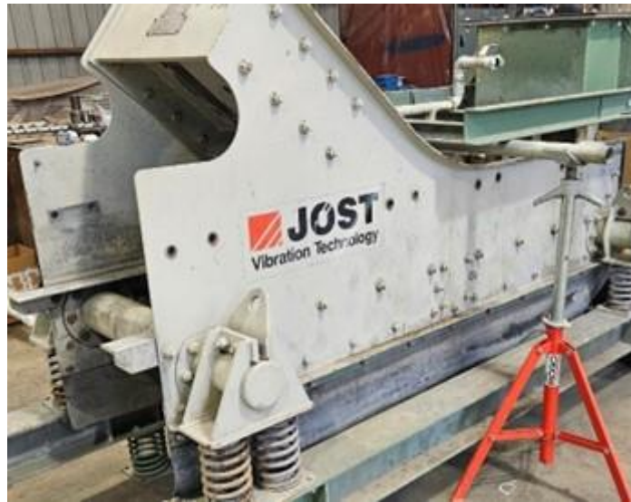
Figure 9: Vibrating Screen and other ancillary processing equipment associated with the Gravity Circuit
