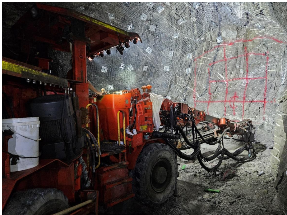
Figure 3: Twin Boom Jumbo advancing the main face of the decline at the 23 Level.
