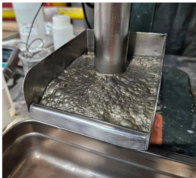
Figure 9: 3rd cleaner sulphide concentrate assaying 29.1% nickel
