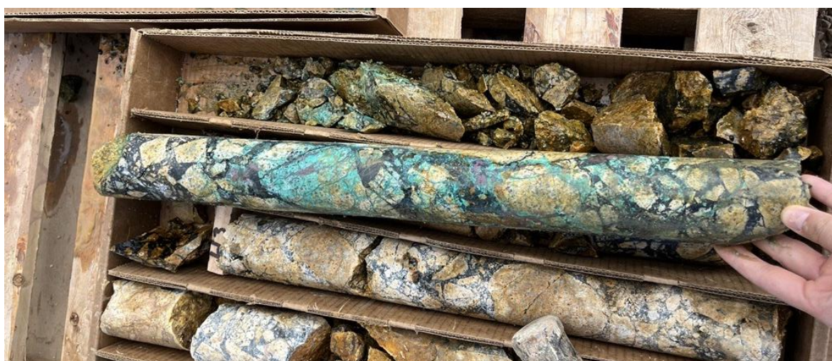
Figure 1: High grade copper mineralisation in tourmaline breccia which contains spot pXRF grades up to 45.5% copper within the interval 14-16m down hole NY2024-DDH2
