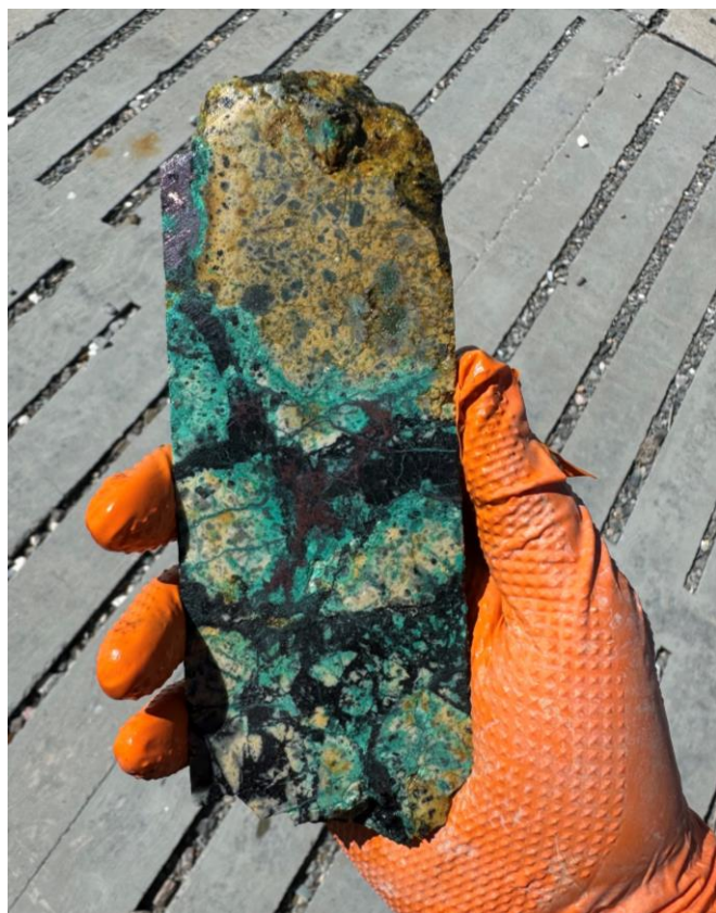
Figure 3: NY2024-DDH2 drill core at 14.0-14.2m downhole. The pXRF copper grade over 3 readings averages 23.2%.
